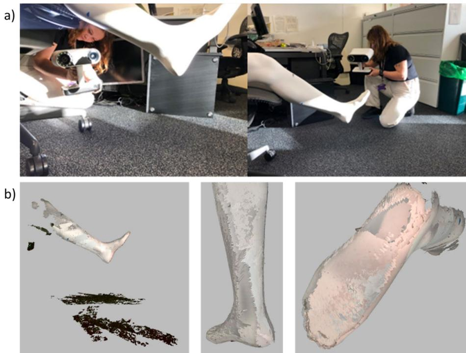
*Figure 3 - a) Artec Leo scanning Prosthetic Lower Limb, b) Raw scanning image from Artec Leo Scans and imported into Artec Studio 16.*
